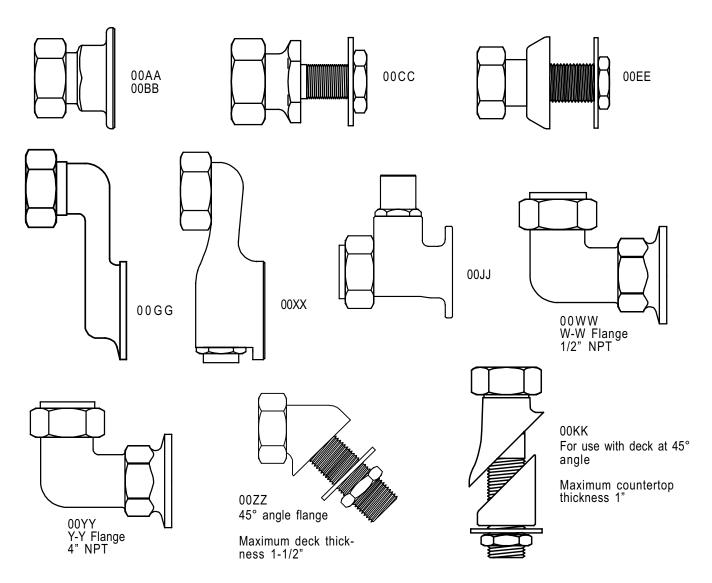
The following inlets are polished chrome plated and used on mixing faucets to meet varying conditions of installation. All are interchangeable and are used in lieu of the "00AA" inlets which are ordinarily furnished on faucets using union coupling inlets. All are available in rough chrome if specified. To order, add suffix letter to faucet model number. For example: "B-0230-CC" sink mixing faucet with 1/2" NPT male inlet, 1" (25 mm) long.
